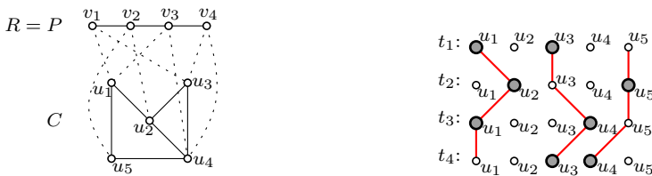
Fig. 1. An instance of the guarding game with the path G[R] and the graph G[C] to be guarded (left). The robber walks on the path G[R] from vertex v_1 in round 1 (layer t_1 ) to vertex v_4 in round 4 (layer t_4 ). Three cops are necessary to guard C , and a strategy of the cops is depicted by the thick lines traversing the vertices of the auxiliary graph which consists of 4 copies of G[C] (right). The highlighted vertices depict vertices on which there needs to be a cop at the respective time.
